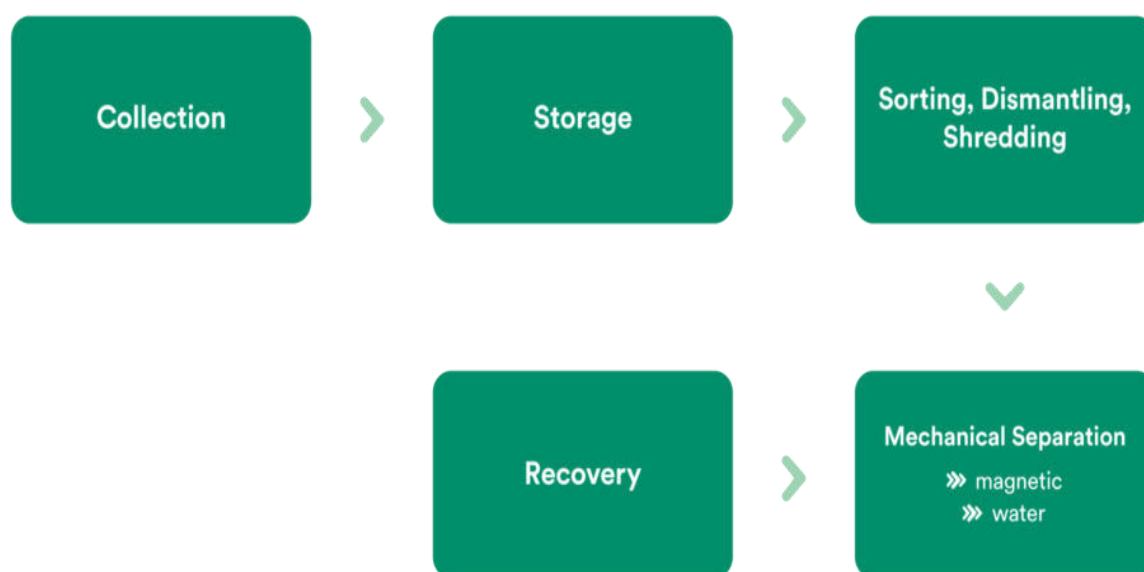
Fig 7 E-waste recycling process flowchart
