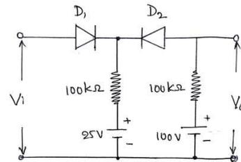
c Write the procedure for analyzing the clamping circuit, determine output voltage for the network shown in fig. (1.b) Assume  $f=1000\text{Hz}$  and ideal diode. 6 Marks
