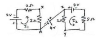
c) If the total power dissipated in the circuit shown below is 18W, find the value of R
