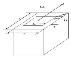
For the body shown in figure, determine the temperature distribution. The body is insulated along the top and bottom edges,  $Kxx = Kyy = 1.7307 \text{ W/m}^{\circ}\text{C}$ . No internal heat generation is
