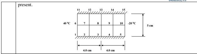
Obtain the temperature distribution for the composite cylinder inside which a hot fluid is flowing, and the outer surface is exposed to surrounding atmospheric conditions as shown. Assume perfect continuity between the layers. Capture the temperature values at the interface of materials (Use an element size of 0.002m or less).
