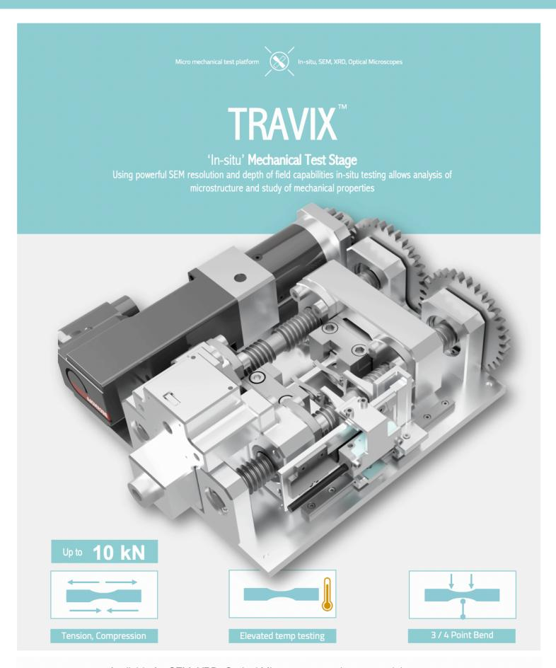
Available for SEM, XRD, Optical Microscopes and as a standalone system
